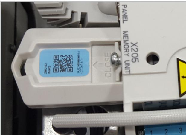
The control parameters and programs are stored on a memory module that is a constituent of the controller.
