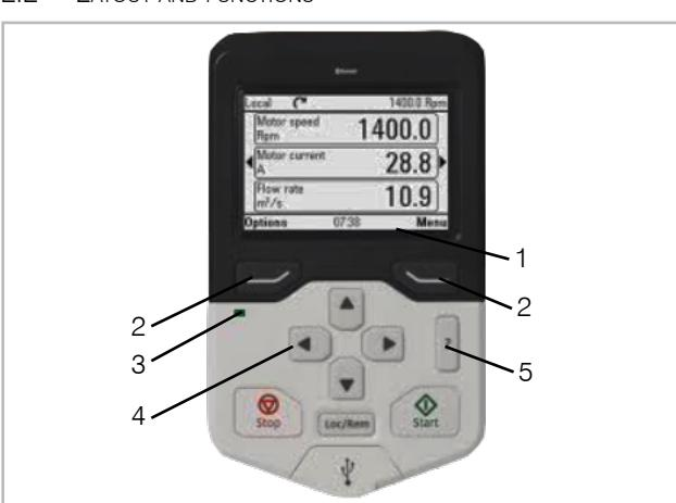
Navigation bar: Shows the current function of the buttons (2) and the time (1). Menu navigation buttons (2). Status lights: green = no fault, red = fault (3). Scroll through menu or list, increase or decrease a parameter value (4). ? button to receive more information in parameters (5).
